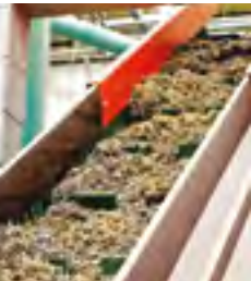
The backing of the carpet is processed into vinyl crumb.
